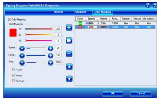
7. In our example we want to mark the green window frames first, so green must be the first color at the top of the list. Normally the color green is the second color down in the list. In order to move it we just select it and press the **Up key** to move it up one position. We now have green at the top and red is the second color down. This is the order in which the colors will be processed.
