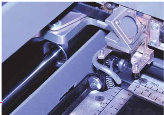
After cleaning the rails and bearings, clean off the table and the rest of the inside of the machine. Spending just a few minutes a week will pay
