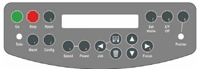
1. To set the IP Address, press the **Go and Pointer keys on the control panel at the same time**. You will see **FUNCTIONS MENU** displayed on the control panel LCD screen.
