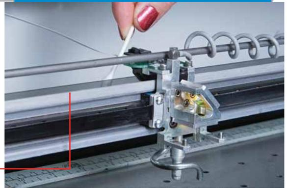
The encoder reader is a horseshoe shaped device that straddles the encoder strip. There is a possibility that dirt and debris can get inside the encoder. Blow some compressed air under the encoder to remove any dust and debris.
