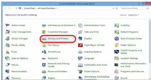
9. In the Unspecified section of Devices and Printers, **right click on the laser's icon**, then click **Properties**.
