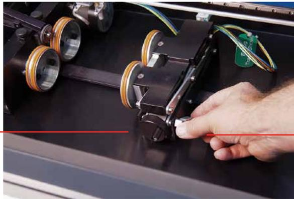
Flip the release lever to move the scissor jack left and right.
